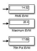
Change the I/Q amplitude imbalance (dB) value in the I/Q Imbalance block to 2 dB. You can see that the all the MER and EVM metrics degrade.
