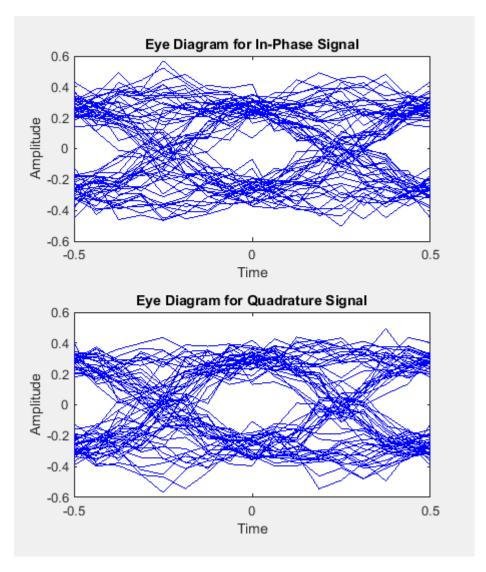
Observe that the received eye diagram begins to close due to the presence of AWGN. Moreover, the filter has finite length which also contributes to the non-ideal behavior.
