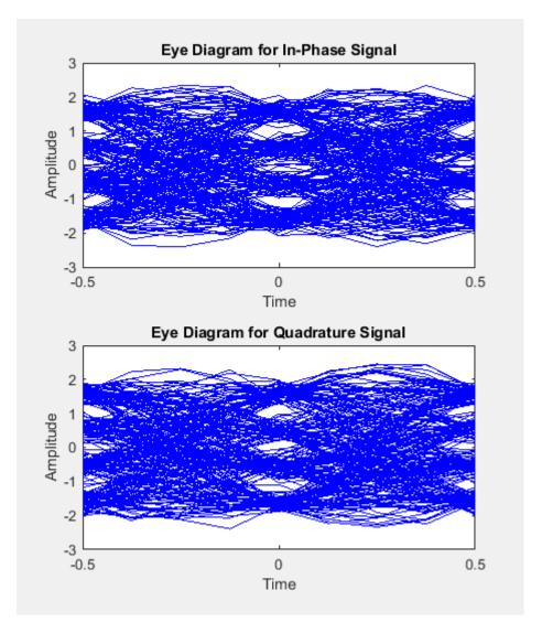
Displaying the eye diagram of the signal after the matched receive filtering is applied shows the signal with raised cosine filtering. The wider eye diagram eye-openings, the signal has less ISI with raised cosine filtering as compared to the signal with RRC filtering.
