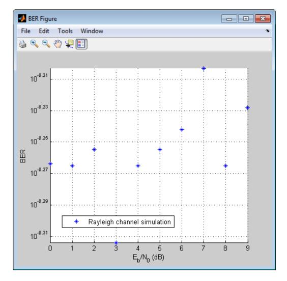
In the presence of multipath fading, the BER performance reduces to that of a binary channel with a consistent value of one-half. To correct the effect of multipath fading, you must add equalization to the communications system.
