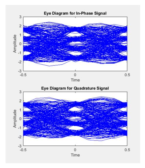
Displaying the eye diagram of the signal after the channel noise shows the signal with RRC filtering and noise. The noise level causes further narrowing of the eye diagram eye-opening.
